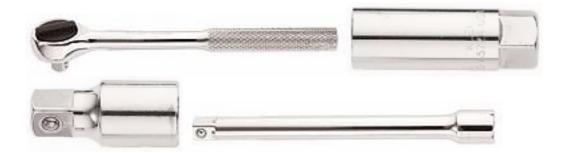
Sockets typically have a square drive hole in one end and a 6 or 12 point opening designed fit various nuts at the other. In the aviation industry the most common size drivers are; <sup>1</sup>/<sub>4</sub>, 3/8, <sup>1</sup>/<sub>2</sub> and <sup>3</sup>/<sub>4</sub> inch. For the AERO1600 course we will use <sup>1</sup>/<sub>4</sub> inch sockets and drivers.
