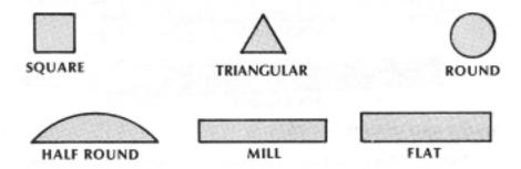
Square files are tapered on all four sides and are used to enlarge square or rectangular holes.
